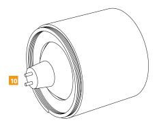
11 Install the diffuser over the bulb, be careful not to cross thread.
